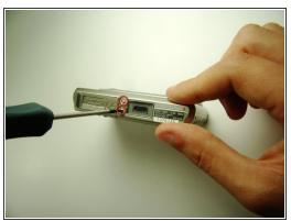
Locate and remove the 3mm screws on the top and sides of the camera with the size 00 screwdriver.
