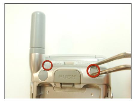
Use a push-pin or tweezers to pry both of the tear-shaped screw covers out of the top of the phone.
