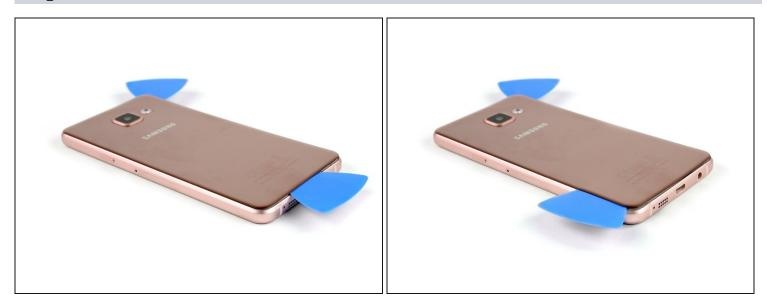
• Insert a second opening pick and move around the other corner at the bottom part of the back cover.
