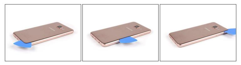
• Slide the opening pick up to the rear camera to separate the back cover from the frame.
