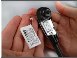
Locate and detatch the white connector that connects the wires of the battery to the wires of the headset.
