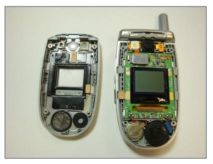
• The case can now be removed and the interior of the front is accessible.
