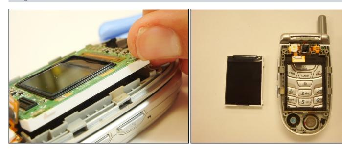
• Remove the main display by lifting up the extruded white edge with your fingernail.
