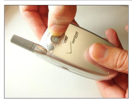
Open the battery casing by pressing the gray "PUSH" button. Slide the back of the casing downward.
