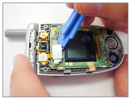
After the solder has been removed, pry off the camera assembly connection shield with the plastic opening tool.
