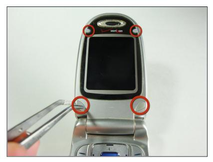
Remove the four grey plugs using either <u>tweezers</u> or a push pin.
