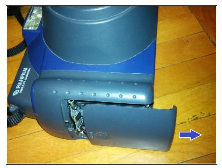
First, push on the recessed part of the battery cover while sliding it away from the camera to remove it.
