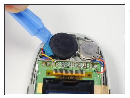
After the solder has been removed, pry out the speaker with the plastic opening tool.
