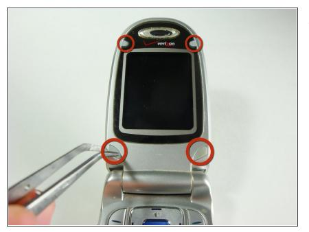
• Remove the four grey plugs using either tweezers or a push pin.
