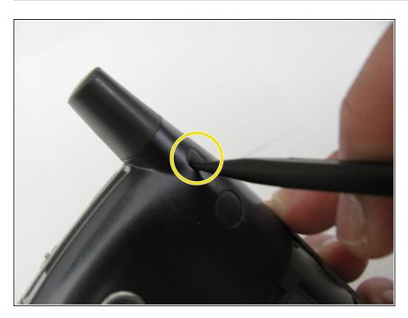
Using the spudger, remove the small rubberized patch under the antenna.
