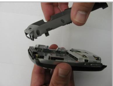
Using the plastic opening tool, gently separate the back case from the phone body.
