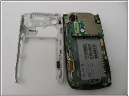
• Using a plastic opening tool, gently edge your way between the back and border case (Picture 2) until they are completely separated (Picture 3).
