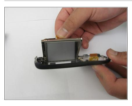
Once the motherboard is removed, the LCD should be resting on the front case of the phone.
