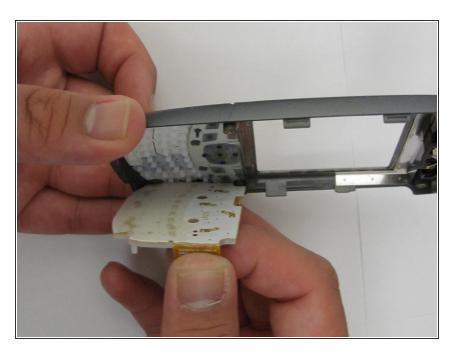
Peel the keypad from the front panel of the case
