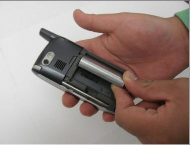
• Use the small notch on the left hand side of the phone to remove the battery.
