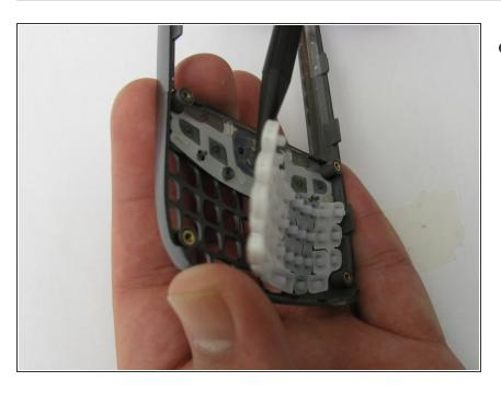
Using a spudger, remove the gel keyboard from the front case.
