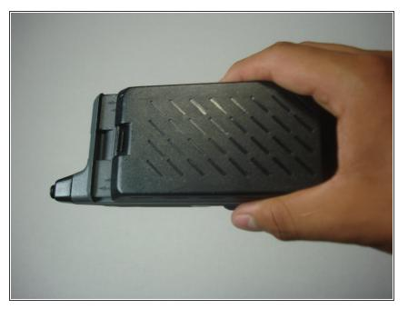
Remove the battery by sliding it down the rails to which it is connected.
