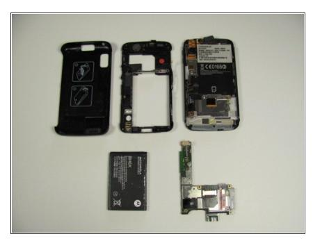
After disconnecting the motherboard, there should be five distinct and separate parts of the phone: back cover, back case, front case, battery, and motherboard.
