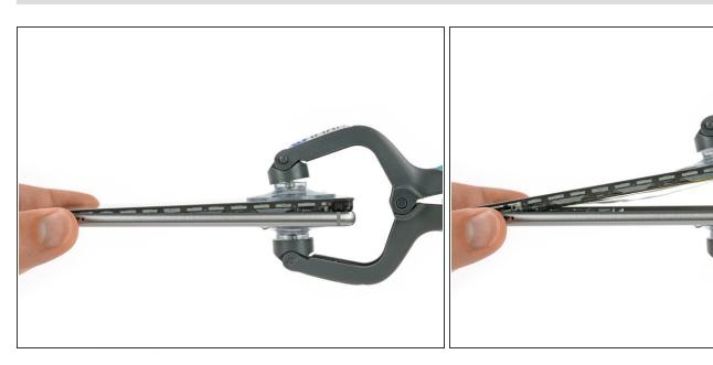
Use an iSclack or a suction handle to separate the display unit from the rear case.
