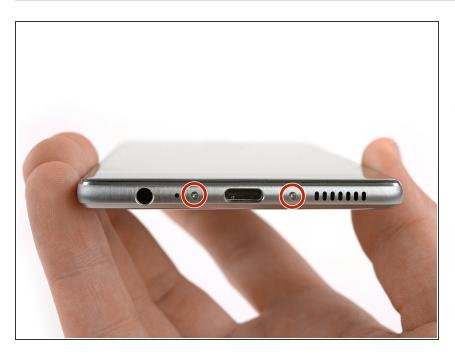
Remove the two P2 Pentalobe screws on either side of the USB C port.
