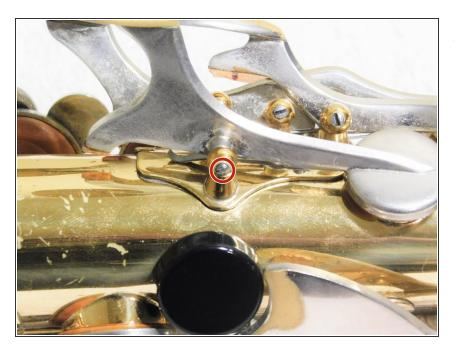
• Screws are located down from key.
