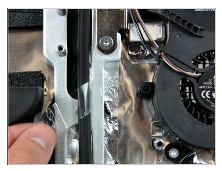
Remove the piece of tape securing the hard drive data cable to the chassis.
