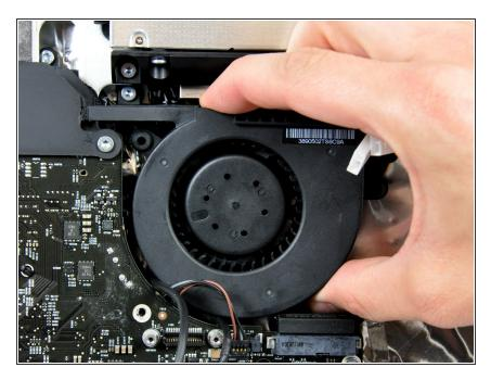
Gently lift the optical drive fan off the plastic posts protruding from the rear case.
