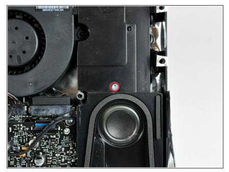
Remove the single T10 Torx screw securing the right speaker to the rear case.
