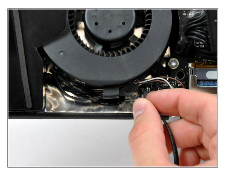
De-route the left fan cable from the channel on the CPU fan.
