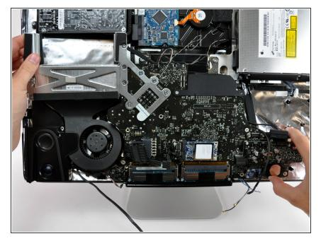
Lift the logic board assembly out of the rear case, minding any cables or I/O ports that may get caught.
