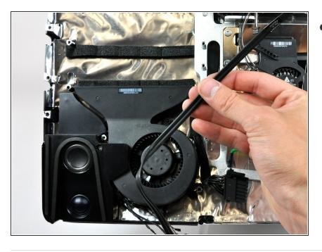
Lift the hard drive data cable out of the rear case.
