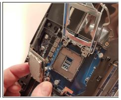
Pull the lever circled in red in the direction of the red arrow while pressing on it.
