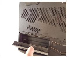
• Lift the battery while unlocking the lock circled in red.
