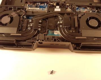
Unscrew the two screws circled in red
