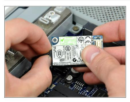
Pull the modem cable connector straight away from the modem. To reassemble your device, follow these instructions in reverse order.
