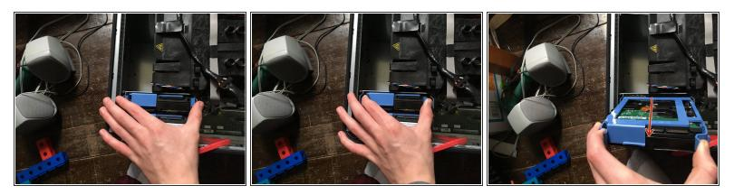
• Pull the two tabs on the hard drive and pull up
