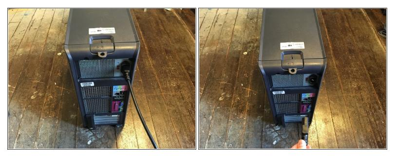
• Power down your PC and remove the power cord from the back.
