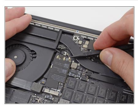
Use the tip of a spudger to detach the three antenna connectors up from their sockets on the AirPort board.
