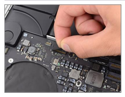
Peel back any tape covering the keyboard ribbon cable connector.
