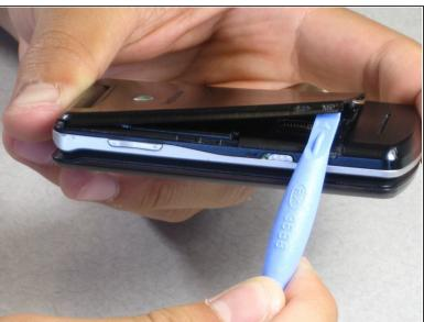
Insert the plastic opening tool in the notch to remove the cover.
