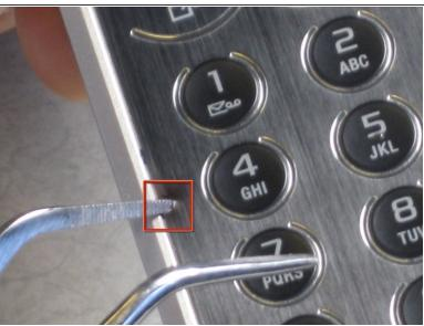
Insert one side of the tweezer into the hole located to the left of the "4" key as shown.
