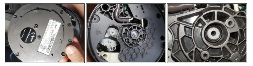
Unscrew 8 screws, remove the bottom cap. find the previous repair of 2 metal washer and take them out. Add a black rubber gasket at the bottom of that stack and put them back on top. It works but not fully. There is one more critical noise fix left; the thin metal arm behind the plastic barrier is making the noise and I cannot reach it easily.
