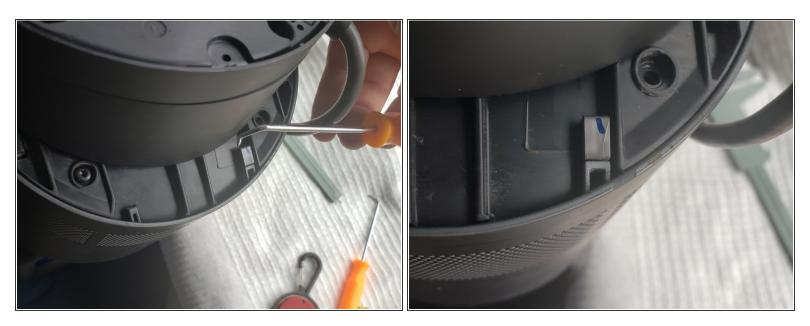
• These pieces that some of us had leftover below on the cover cap. So go back to step 1, remove remove the 4 screws in the intermediate stage (not the bottom 6 screws). SLIGHTLY lift up the cap and slide the plastic part horizontally along the cap into place. The push the cap back down and tighten the 4 screws back into place.
