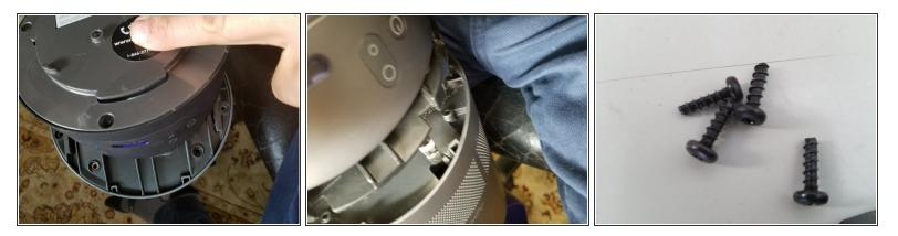
• Turn the Dyson upside down, there are 6 to unscrew. If you only see 4 screws, slide the fan back the other way to reveal 2 on the other side.
