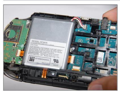
Once the ribbons have been removed, then the back is fully removed and you can access the hardware within.
