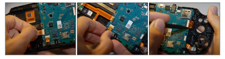
Next you must remove the two ribbon cables connecting the motherboard to other hardware parts. Please be **careful**. The third ribbon on the bottom is a camera that also needs to be carefully removed.
