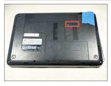
Locate the lock switch on the bottom of the computer.
