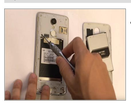
Remove the ten screws with a Phillips #00 screwdriver.
