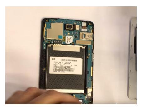
Use finger nail or wedge to gently remove dust cover, and reveal the motherboard.
