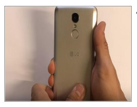
Remove back plating to expose the battery, sim card, and SD card (if applicable)
