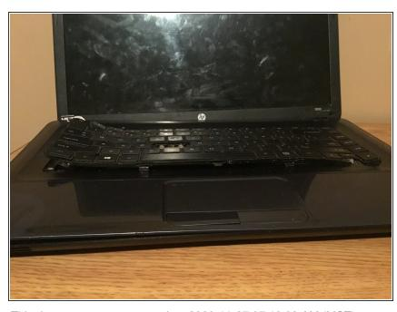
My keyboard is kind of bad so the general idea is to get a flat bladed screwdriver under Neath of the old keyboard not the keys it may help if you take all of the old keys off around the sides
