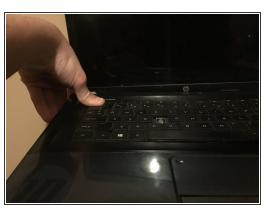
Put the pins of the new keyboard in then put it back into place as the old one was.
