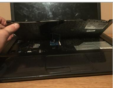
pry Up on the old keyboard until you see the 5 pins pop up out of place once all 5 come undone the old key board should come right out
