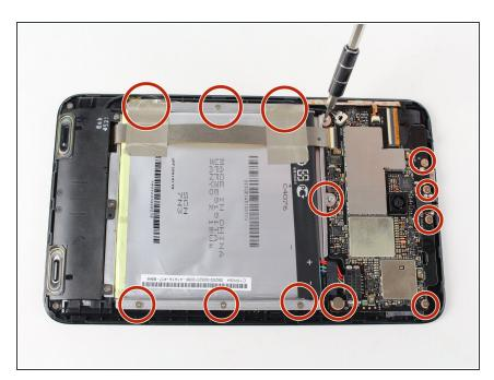
Remove the screws (2.6mm) connecting the motherboard and battery tray to the hard frame with Phillip's head screw driver (PH000).
