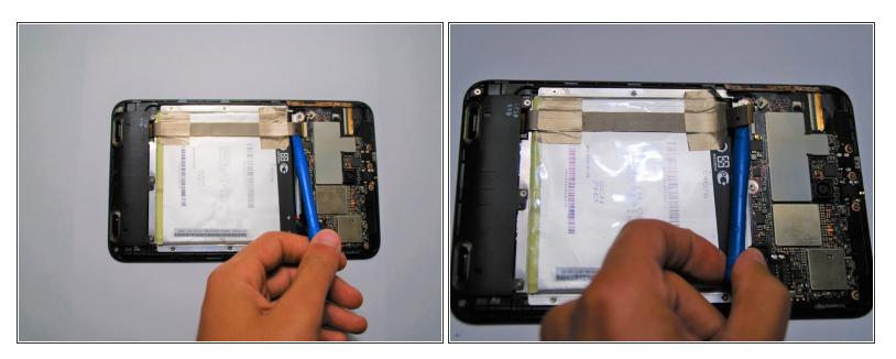
• Use plastic opener tool to disconnect ZIF connectors as shown.
