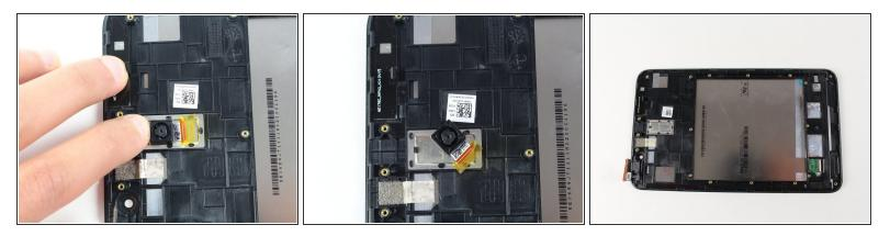
• Apply slight pressure on camera to break adhesive to finish screen disassembly processes.
