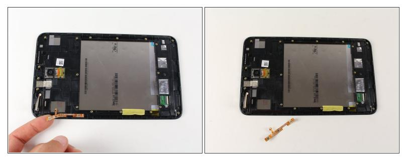
• Peel off button sensors off the side of the hard frame.
