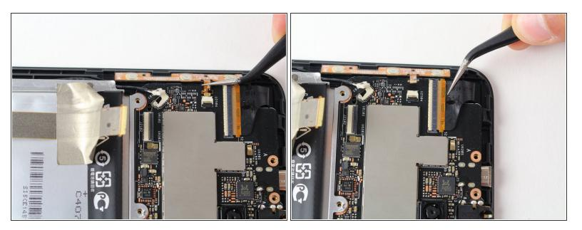
• Remove display and button connections from motherboard using metal tweezers.
