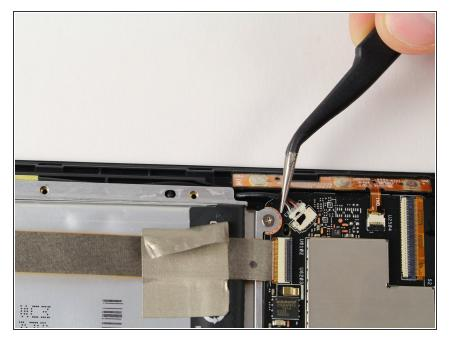
Disconnect speaker wire from motherboard using metal pronged tweezers.
