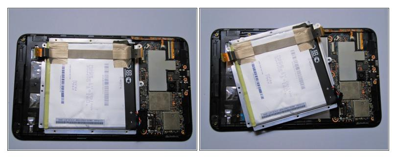
Remove unscrewed battery tray from main frame.
