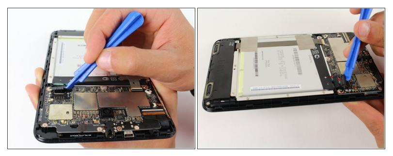
• Remove the black bundle battery connector from the motherboard using plastic opening tools.
