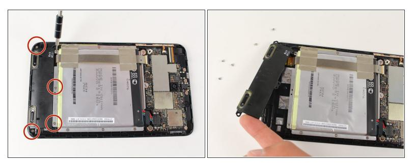
Remove screws (2.6mm) connecting speaker to hard frame with Phillips head screw driver (PH000).
