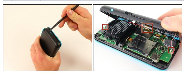
A Be careful when separating the bottom panel from the front casing to avoid breaking the three cables connected to the motherboard (two on each side and one in the rear).
