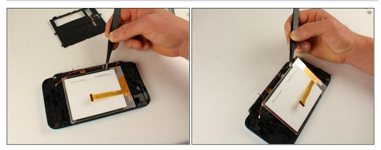
A The bottom screen is stuck to the front with an adhesive border. Be careful to slowly separate the two. Quick separation can damage both components.
