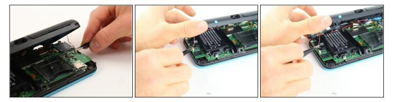
• Using tweezers, disconnect the two cables that connect the rear buttons on either side to the motherboard by gently pulling them upwards.
