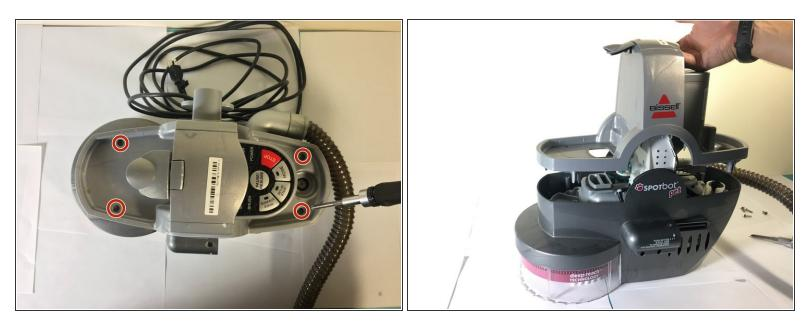
Unscrew the 4 screws on the top of the device and gently lift the top half up.
