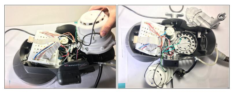
• Lift the white suction motor from the right side of the device. Lift it straight up and set it off to the side of the vacuum.
