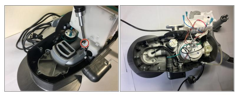
• Unscrew the screw next to the white plastic wiring harness box. This will then allow you to set the white box off to the side.
