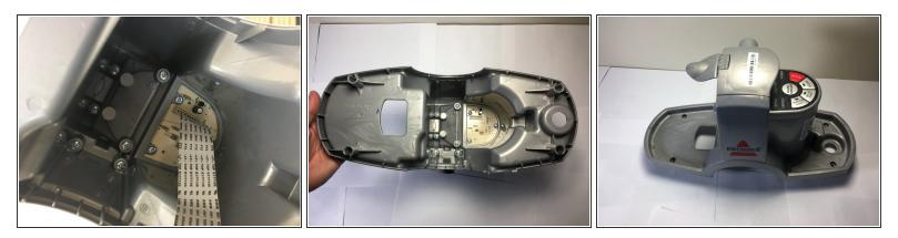
Unplug the ribbon cable that connects the bottom half to the control panel on the top half. Then, set the top half off to the side.
