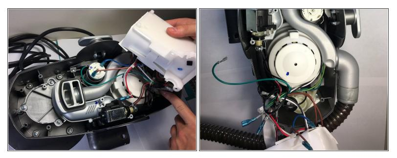
• Unplug the wires by disconnecting the section that connects the motor to the wiring harness.
