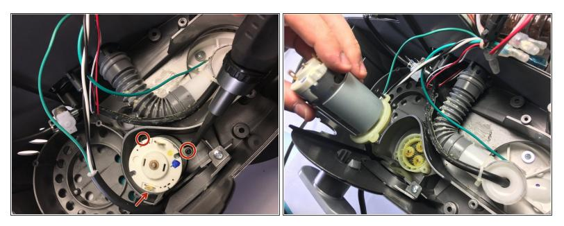
Unscrew the screws for the brush motor as shown, this motor controls the automatic scrubbing mechanism.
