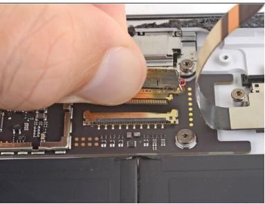
Slide the SurfaceConnect port connector out of its socket on the motherboard.
