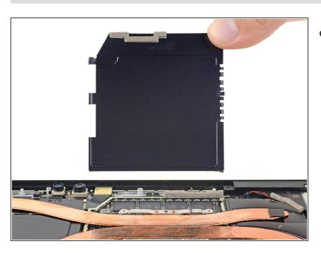
Remove the heat sink shield.
