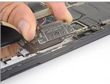
Gently pull the SurfaceConnect port out of its recess in the case and remove it.
