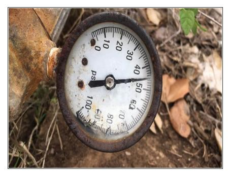
Here is a time lapse of what the pressure gauge showed. The pressure switch did not cutoff and rising pressure caused some faucets to develop leaks.
