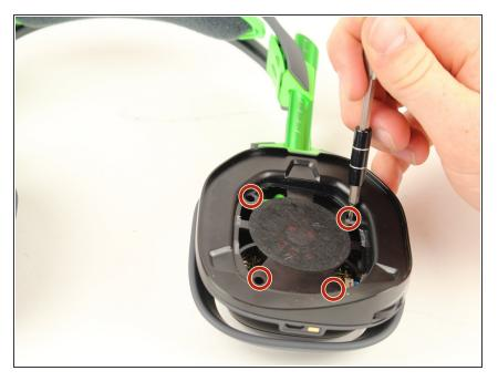
Remove the four 6mm Phillips 1 screws.
