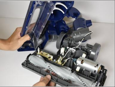
Lift the grey frame off the bottom of the vacuum cleaner with your hands and place it on a flat surface.
