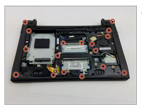
Unscrew the circled screws, a total of 17 (15 M 2x6 and 2 M 2x3), with a cross-head screwdriver.
