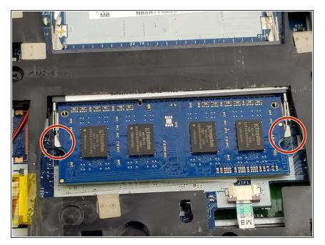
Locate the RAM and the metal clips holding the RAM in place.
