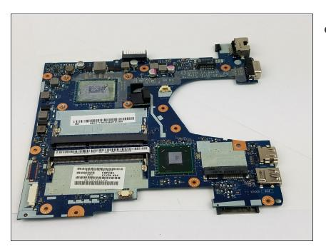
• The motherboard is now bare of any extras and is ready to be replaced.
