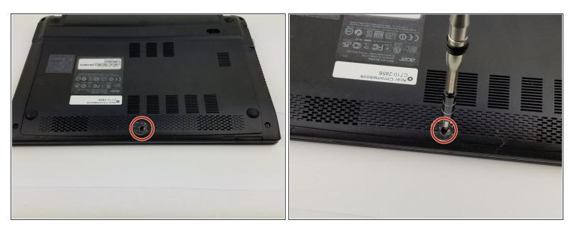
• Remove the one 4.3mm Phillips #1 screw holding the back cover on.
