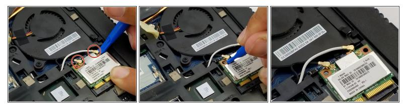
• Use the blue plastic opening tool and carefully remove the connectors from the Wi-Fi card.
