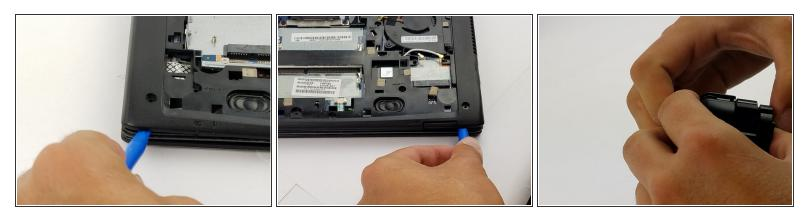
• Using the blue plastic opening tool, work your way around the perimeter of the laptop and remove the bottom frame.
