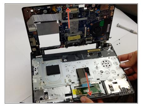
Now completely pull apart the motherboard from the underside of the laptop by pulling on the location of the arrows.
