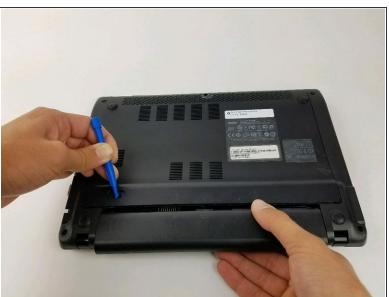
On the underside of the laptop towards the back, locate the battery lock slider. Push the slider, and remove the battery.
