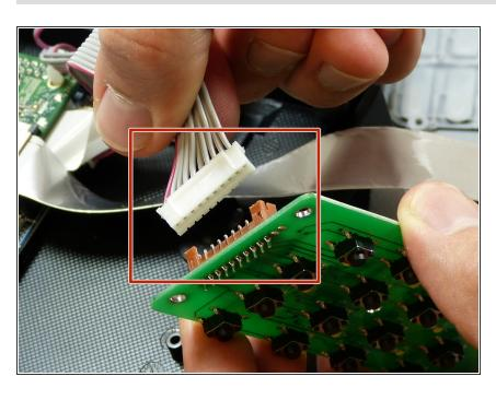
Remove the bundled cable connector from the keyboard by pulling the cable away from the connector in the same direction as the individual wires are running. To reassemble your device, follow these instructions in reverse order.
