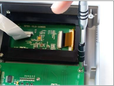
Remove the five 7mm PH #1 screws from the back of the keypad, by rotating the screw driver counter clockwise, removing the screw from the housing completely.
