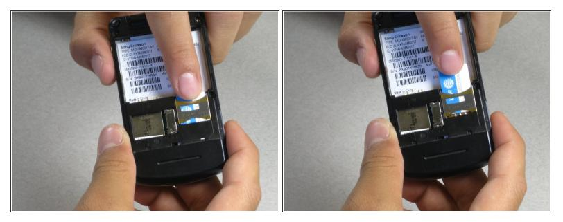
• Using you finger to pull out the SIM card.
