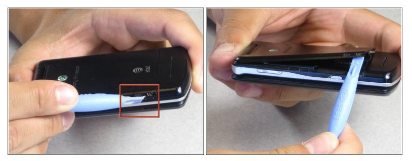
• Insert the plastic opening tool in the notch to remove the cover.
