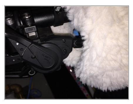
On the lefthand side of your Stromer, bend over to have a look below the gear shifter. Notice it has a switch. First take note of the position of the switch and flick it to the other side. Try again and see if your problem has been fixed.
