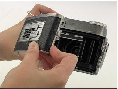
• Lift the back cover away from the camera in order to free the latch on the left.
