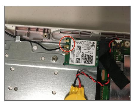
Disconnect the two wires that are connected to the Wi-Fi card by gently pulling them up.
