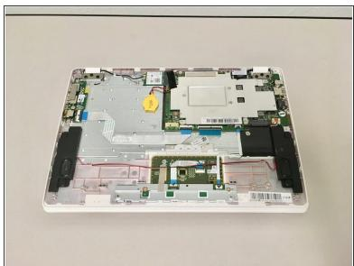
Lift the battery up and out of the device.
