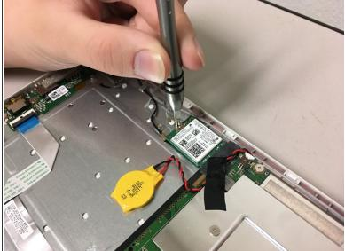
• Unscrew the one 4mm screw keeping the card in place.
