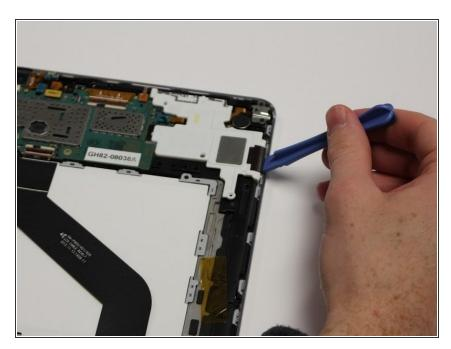
Remove the white cover over the audio jack with the plastic opening tool by pushing up on the black connecter.
