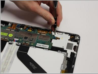
• Remove the two 3mm Phillips #00 screws securing in the white cover over the audio jack.
