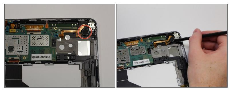
Pull up on the circular amp with the spudger tool to release it from the device.
