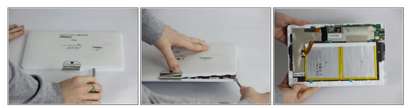
• Using the metal spudger, carefully pry open the back cover.
