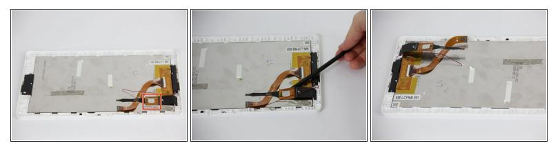
• Using a plastic spudger pry the square connection away from the screen.
