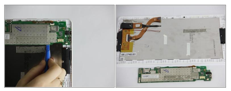
• Using the small plastic tool, carefully pry the motherboard out of the device.
