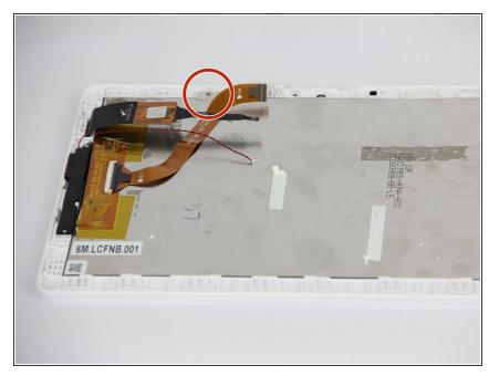
• Using the Philips #00 head unscrew the screw holding in the small plate.
