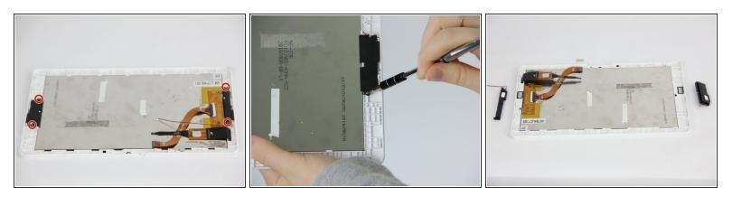
Using the Philips #00 unscrew the remaining 4 screws along the two speakers.
