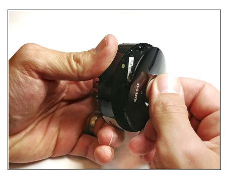
To remove the front cover, place index finger in the center and pull away from the frame. This may take a little effort, but should not require an opening tool.
