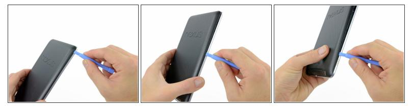
Pry up the rear panel along the left edge using the method described in previous steps.
