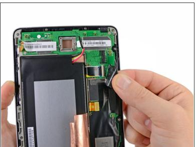
Carefully peel back the adhesive tape covering the I/O board ribbon cable socket on the motherboard.
