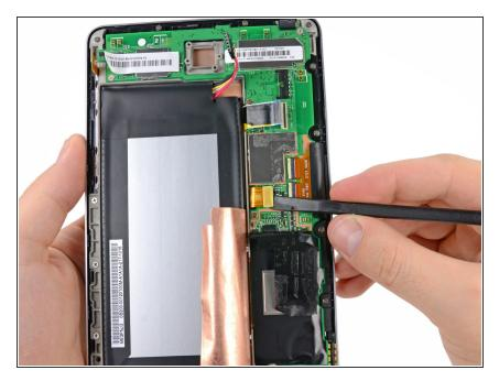
Use the flat end of a spudger to pry the display data cable straight up off its socket on the motherboard.
