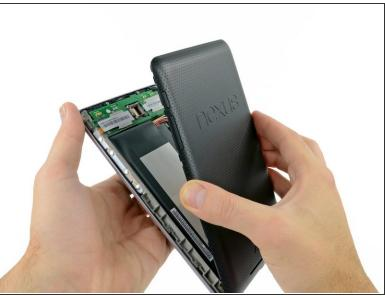
Gently lift and remove the rear panel up off the front panel assembly.
