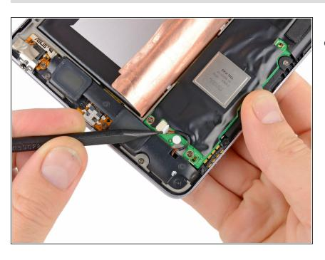
Using the tip of a spudger, push the speaker cable straight out of its socket on the motherboard.
