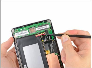
• Using the tip of a spudger, push first on one side then the other to "walk" the battery cable straight out of its socket on the motherboard.
