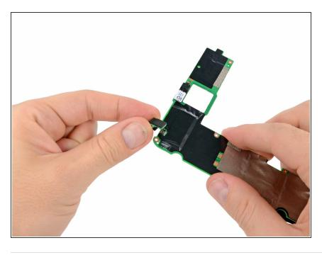
Gently pull the upper microphone straight up off its socket located on the back of the motherboard.
