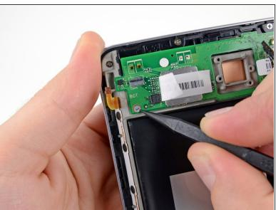
Use the tip of a spudger to remove the warranty seal stickers.
