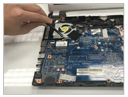
• Disconnect the two wires connected to the Wi-Fi card.
