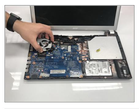
• Carefully remove the CPU fan.
