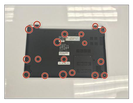
Unscrew the eighteen 8 mm Phillips #0 screws attached to the laptop.
