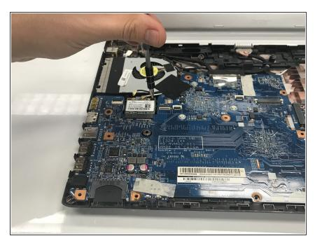
• Unscrew the two 8mm Philips #0 screws attached to the Wi-Fi card.
