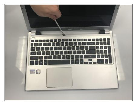
• Pry open the keyboard at the top of the keyboard.
