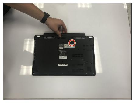
• Unlock the battery by pushing the button to the right.
