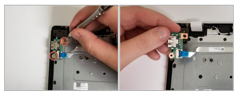
Remove the two screws holding down the USB Port.
