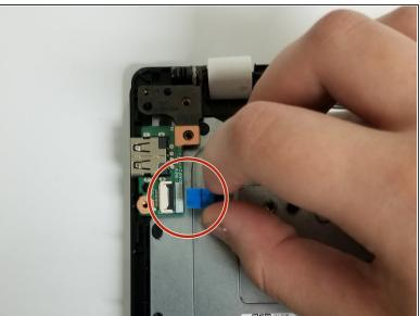
Now that the port can be lifted up, remove the ribbon cable by using the sticker attached to it.
