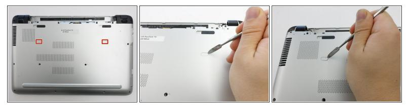
Remove the two plastic tabs with a metal spudger.
