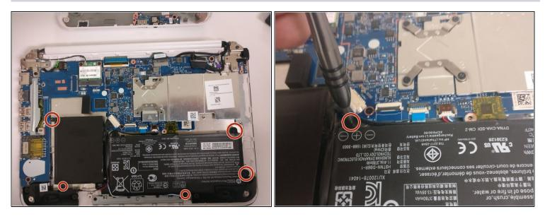
Remove the five 1 mm screws connecting the battery to the base of the computer using a Phillips #0 screwdriver.
